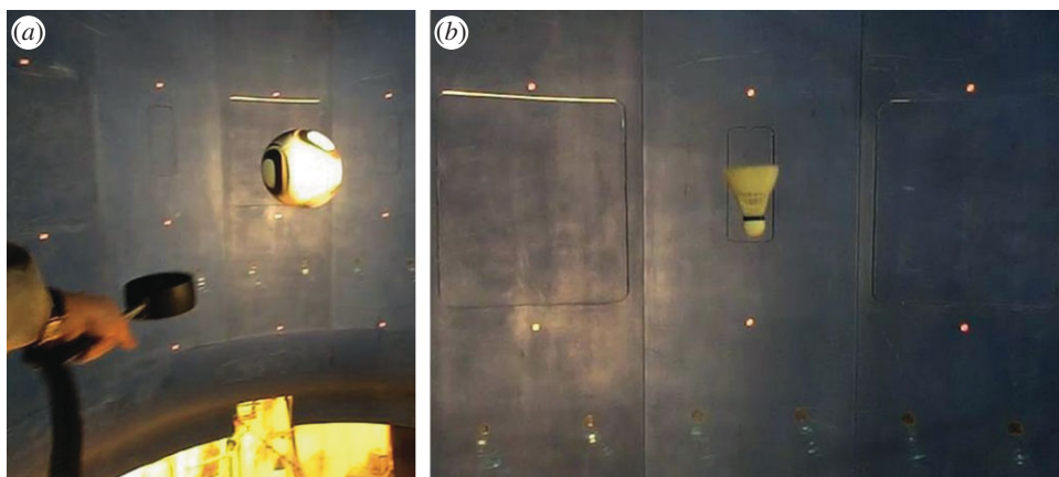
Figure 4. Terminal velocity measurements performed in the vertical wind tunnel SV4 of ONERA-Lille: (a) levitating Jabulani soccer ball at U_\infty = 30 \text{ m s}^{-1} ; (b) levitating feather shuttlecock at U_\infty = 6.7 \text{ m s}^{-1} . (Online version in colour.)
