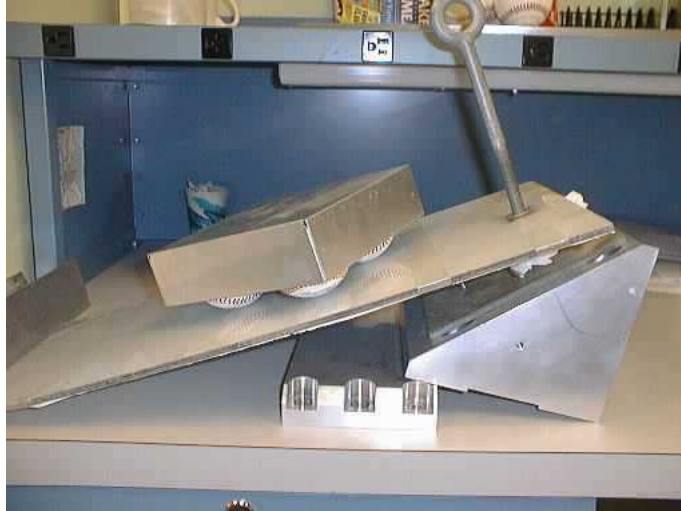
Figure 3. 4-Ball Friction Test Set-up
