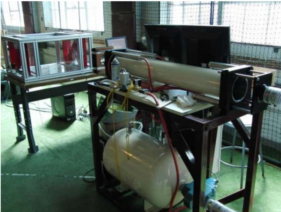
Figure 4.3 - 1st light box and pneumatic cannon
