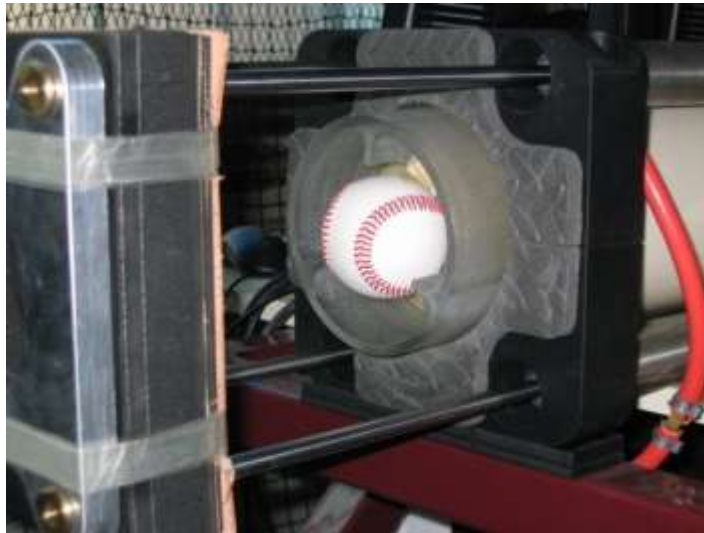
Figure 4.5 - Sabot placed in the cannon's barrel.
