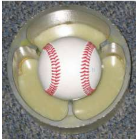
Figure 4.4 – Baseball loaded into the polycarbonate sabot.
