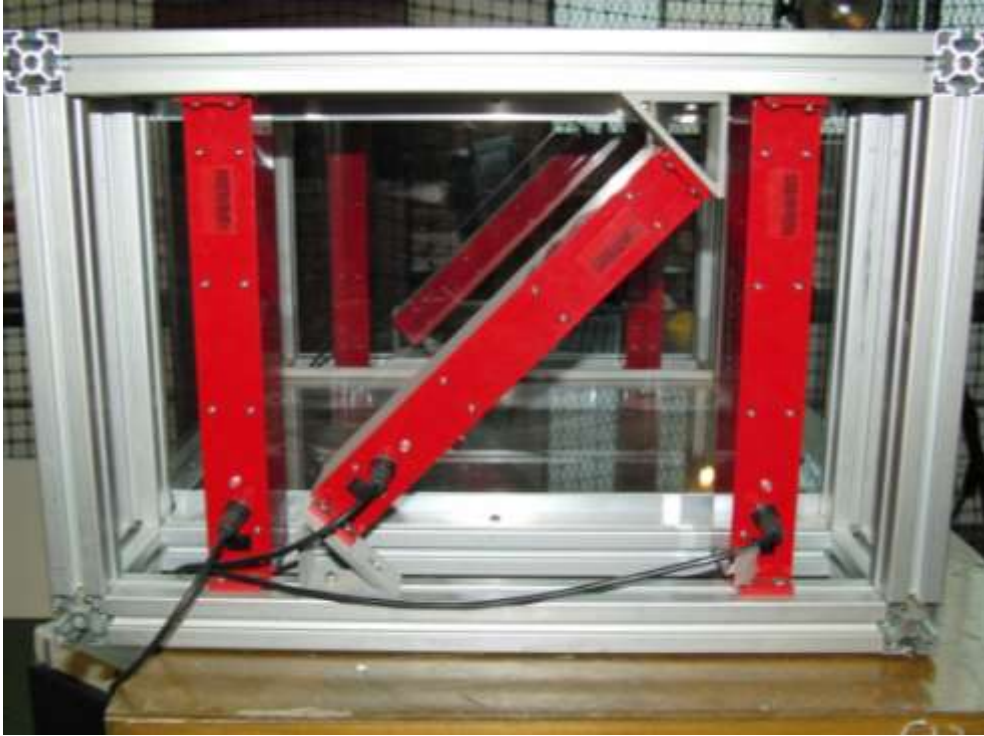
Figure 4.1 - Light gates configuration inside the light box.
