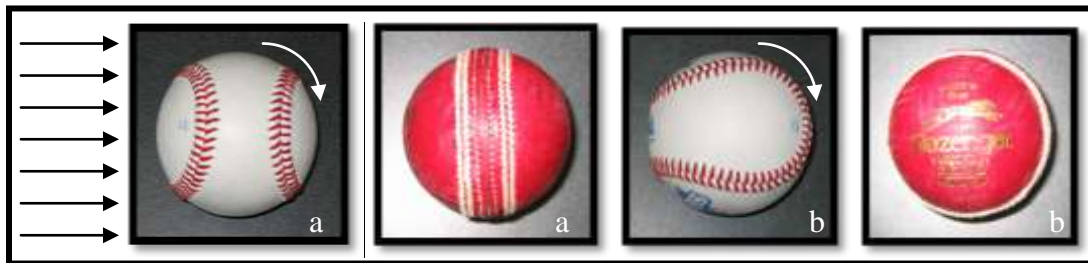
Figure 4.25 - Diagram showing the normal/4-seam (a) and parallel/2-seam (b) orientations. Black arrows indicate the airflow direction, white arrows indicate the ball rotation axis.
