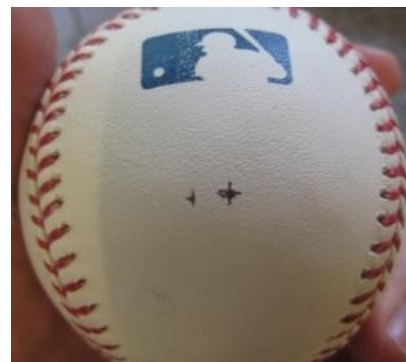
Fig. 2-2: A picture of a Major League Baseball where the two-seam axis of rotation is found. The “+” is the final, corrected point where the other mark is the initial point.
