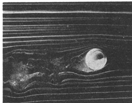
FIG. 1. Showing airflow past spinning ball in wind tunnel. Wind coming from right, 60 ft/sec. Spin 1000 rpm, counterclockwise, about a horizontal axis at right angles to wind. Magnus force, upward. Courtesy of Professor F. N. M. Brown, University of Notre Dame.
